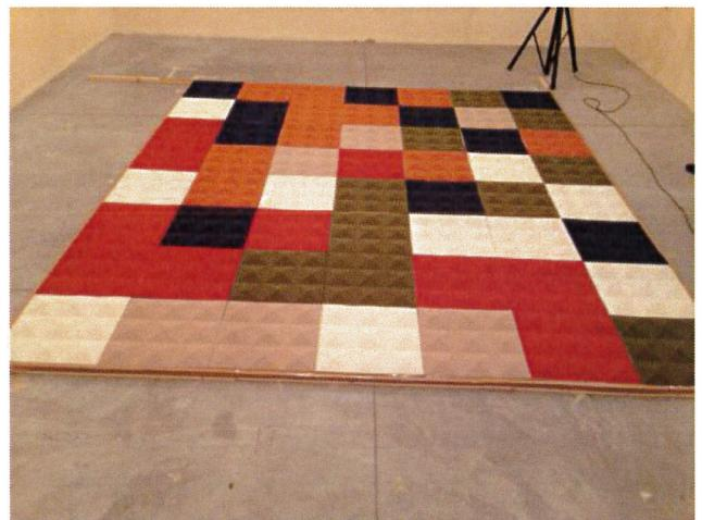
**Test specimen description:** panel mod. "STILLY" (nominal size 440 mm x 440 mm, maximum height 40 mm, mass 0,4 kg) composed of a plastic support frame and polyester felt (6 mm thick) lined with Trevira polyester tissue. Cavity with expanded polyurethane panel (thickness 25 mm, density 30 kg/m<sup>3</sup>).
